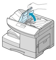
**2** Squeeze the tab at the bottom of the ADF rubber assembly and then pull it out.
